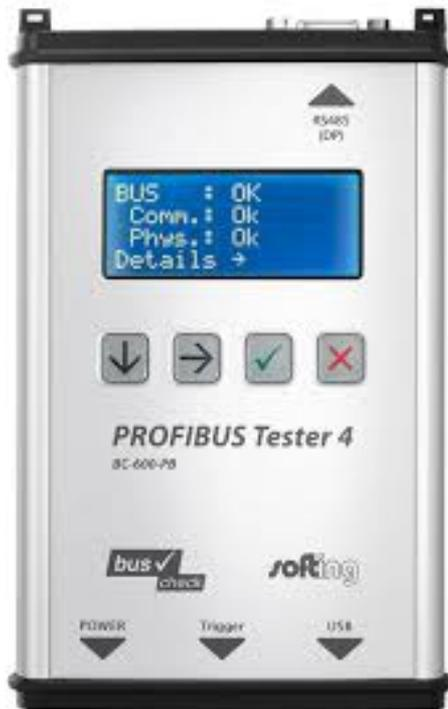
Imagen 4.1.3: Profibus tester, Softing, Tester 4
