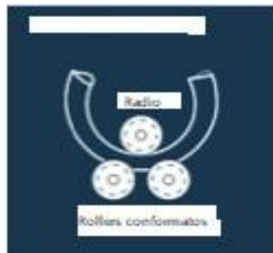
Figure 6 Bent by rollers
